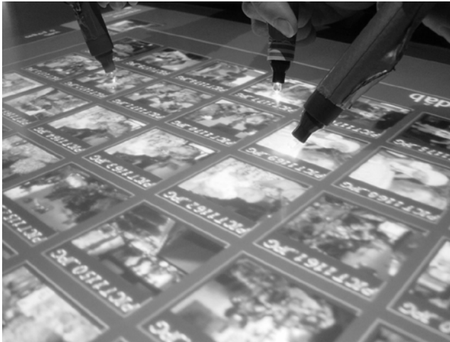
Figure 6: The MultiLightTracker [11] technique in use on a MediaTable
